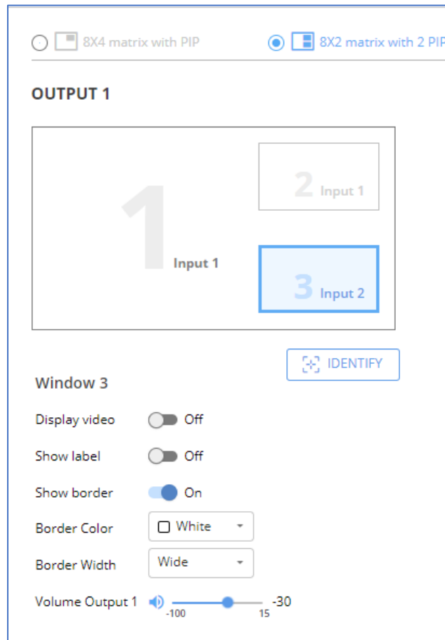
Figure 37: 2 PIP (8X2 Matrix) Layout – – Window 3 Parameters Settings
