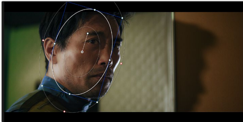
Power windows let you make secondary corrections to specific parts of your image
