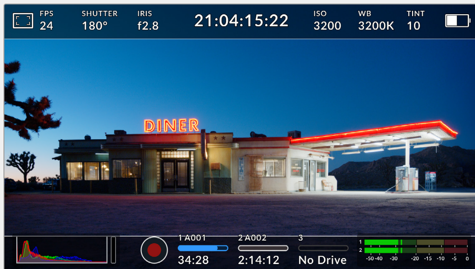
The LCD touchscreen with 2.40:1 frame guides enabled
