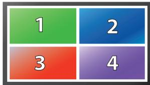
**Quad-Mode** - In Quad mode, the screen is split into four fields of equal size with the screen content of four video sources or computers being displayed in each of these fields. Keyboard and mouse operation can be selected to the field of the corresponding computer.
