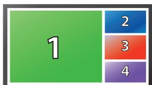
**PiP Mode** - In the PiP(picture in picture) mode, the full screen display of one of the four video sources is accompanied by one or three small images (thumbnails) containing the other video sources on the right-hand margin of the screen allowing simultaneous monitoring.
